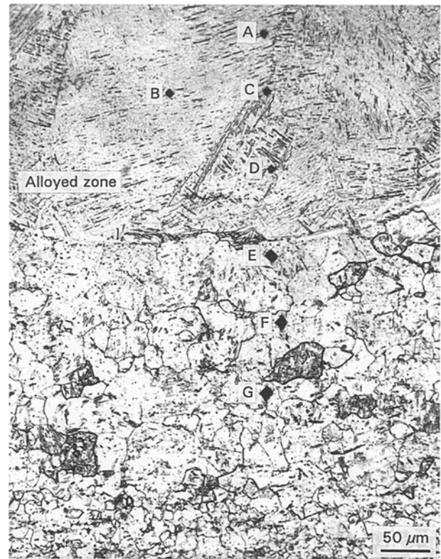
Figure 4 Microhardness measurements within and outside the laser surface alloyed layer (A, H_v , 368; B, H_v , 392; C, H_v , 380; D, H_v , 412; E, H_v , 184; F, H_v , 161; G, H_v , 143).
